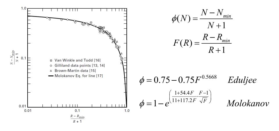
The FUG method is not able to provide us any information about the optimal feed tray: short-cut correlations can be used for this purpose.
