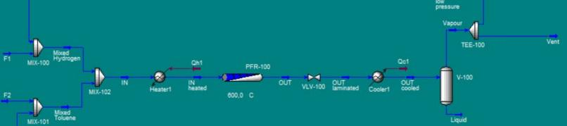
Split the vapour stream according to the Split Factor from MATLAB
