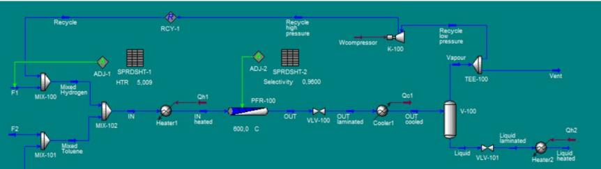
Laminate the liquid stream to 3.6 bar and heat it up to 93.35°C
