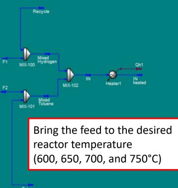
Toluene Recycle **Reaction section**
