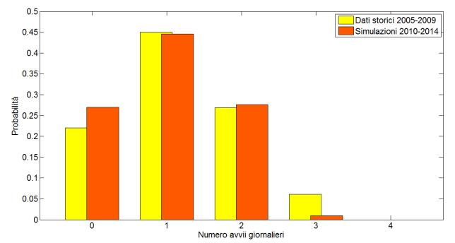
• It is worth observing how the EPS should be switched on (and consequently off) a maximum of 3 times per day. In addition there is a good agreement between the historical data (yellow bars) and the five-year simulations (orange bars).
