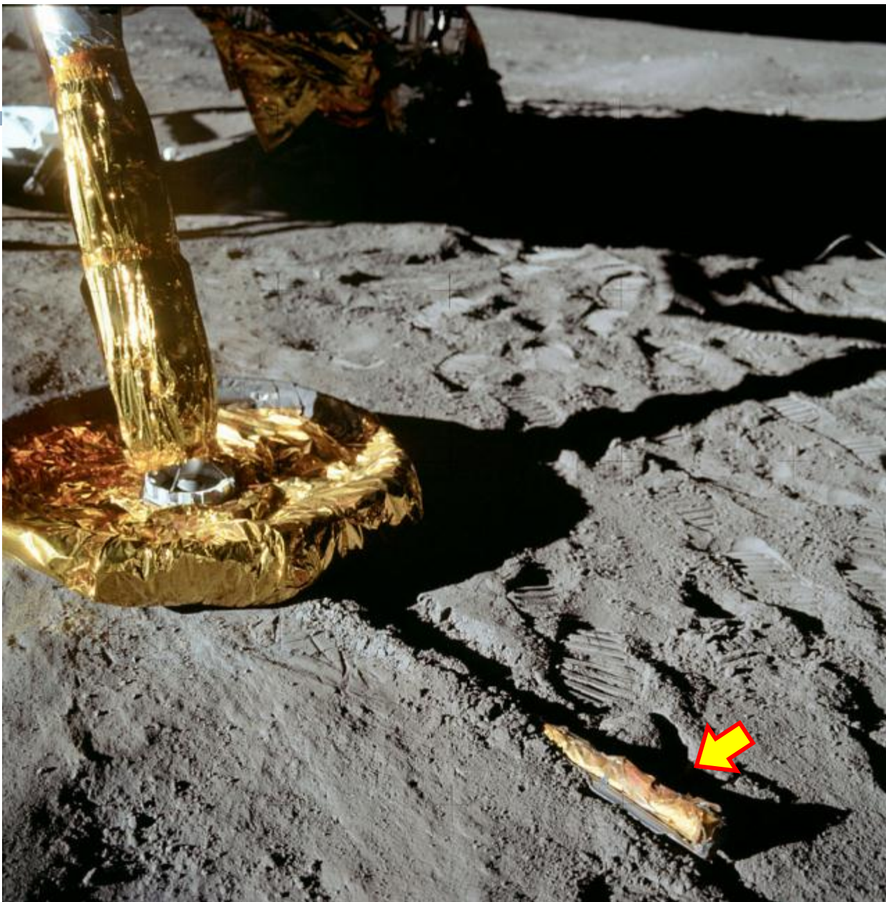
LM footpad and contact probe. Kapton and Mylar-foil from DuPont (16 layers), -150^{\circ} + 130^{\circ} \text{ }^{\circ}\text{C}
