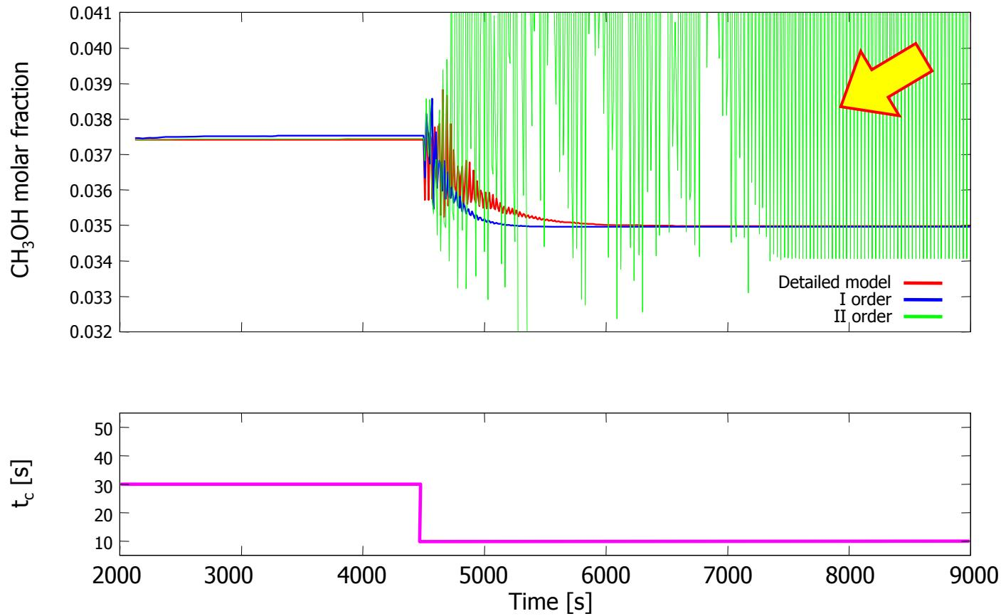
Disturbance on the **switch time** (from 30 to 10 s)
