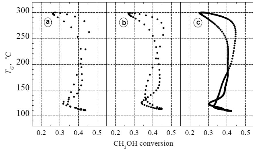
Fig. 6. Correlation between methanol conversion and the outlet gas temperature for different switching times. (a) Period =  $47 t_c$ ,  $t_c = 20$  s; (b) period =  $72 t_c$ ,  $t_c = 22$  s; (c) period =  $332 t_c$ ,  $t_c = 24$  s. Points are taken in the middle of each cycle.
