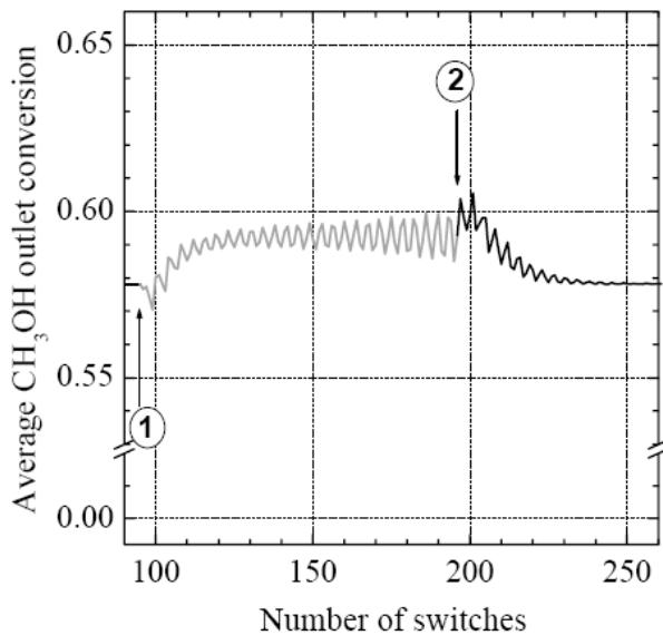
Fig. 8. Open loop response to a step disturbance  $\Delta T_{G,\text{in}} = -10^\circ\text{C}$  (point 1) and restoration of the previous steady-state after the disturbance (point 2);  $t_c = 40\text{ s}$ ,  $T_{\text{in}} = 130^\circ\text{C}$ .
