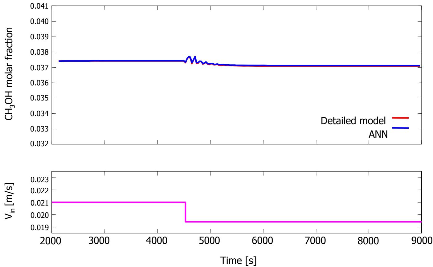
Disturbance on the **inlet velocity**  $0.021 \rightarrow 0.0194$  [ $\text{m/s}$ ]
