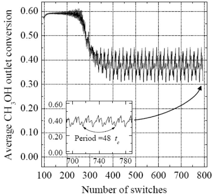
Fig. 7. Open loop response to a step disturbance  $\Delta T_{G,\text{in}} = -10^\circ\text{C}$  and transition to a multi-periodic steady-state;  $t_c = 40 \text{ s}$ ,  $T_{\text{in}} = 130^\circ\text{C}$ .
