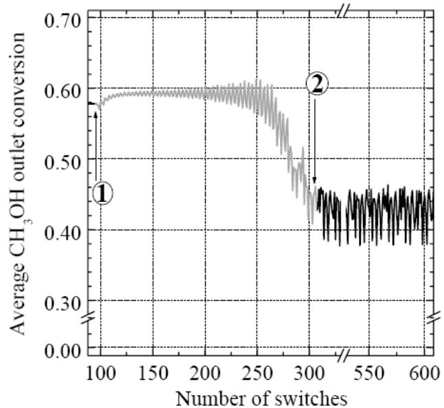
Fig. 9. Open loop response to a step disturbance  $\Delta T_{G,\text{in}} = -10^\circ\text{C}$  (point 1) and new complex steady-state obtained when the conditions before the disturbance are restored (point 2);  $t_c = 40\text{ s}$ ,  $T_{\text{in}} = 130^\circ\text{C}$ .
