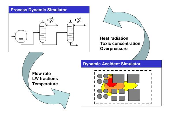
AXIM<sup>™</sup> is a dynamic accident simulator that can be either linked to a process dynamic simulator by means of **OPC** protocol, **DLL**, **OBJ** or work as a standalone package
