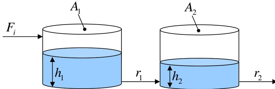
$$\begin{cases} A_1 \frac{dh_1}{dt} = F_i - \frac{h_1 - h_2}{r_1} \\ A_2 \frac{dh_2}{dt} = \frac{h_1 - h_2}{r_1} - \frac{h_2}{r_2} \end{cases}$$
